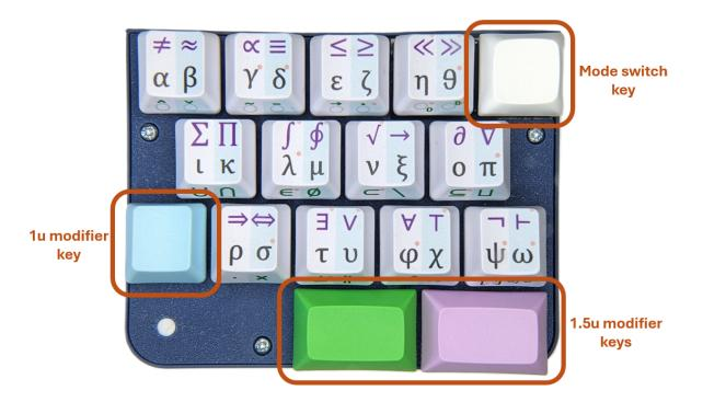
The most challenging aspect of building your own Mathboard is getting the symbols onto the 12 symbol keys. This is done by UV printing, which prints the symbols onto the keys with special UV-curing ink. A UV printer is expensive and requires regular maintenance, so it is not a common device. You may be able to find one if you inquire with local makerspaces, fab-labs, or printing services.
